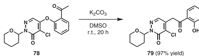
Scheme 27. Example of successful rearrangement of 4-pyridazinyl substrate. 46
