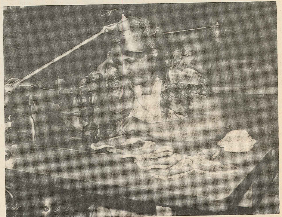
Walking-Foot machine operator Louise Small Legs explains that in an effort to avoid wastage, the trim and vamps are sewn together to form a continuous chain.
