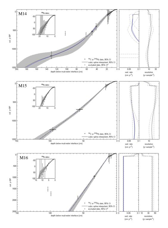
**Figure 4:** Age-depth models for the eight lakes. The main figure shows the age-depth model based on the <sup>210</sup>Pb and <sup>14</sup>C isotope dates. The two sub-figures on the right show the sediment accumulation rate and corresponding sample resolution. Note the different scales on the axes. All age-depth modelling was performed using the MCAgeDepth computer program (Higuera 2009).
