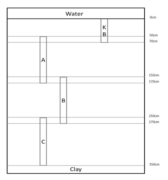
**Appendix X:** Theoretical sampling procedure for extracting successive sediment cores from the lake bottom. The Kajack Brinkhurst core is depicted as KB and the Livingstone cores are depicted as A, B, and C. During field sampling the 20 cm overlap is to enable merging the cores into a single continuous record.
