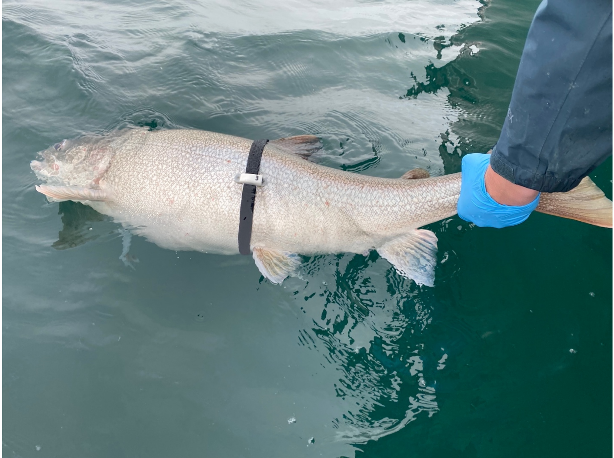
Plate 3.2 Placement of a tri-axial accelerometer harness on a lake trout ( Salvelinus namaycush ) to quantify behaviour following angling. The accelerometer was bonded to a waterproof 3D-printed plate using marine epoxy and then threaded onto a section of Velcro tape that was fastened anterior to the dorsal fin with the accelerometer on the lateral side above the left pectoral fin.
