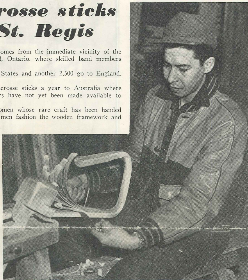
SKILLED WORKMEN: Walter Delorme, goalkeeper of St. Regis Lacrosse Team, is a "stick man" or "knife man," one of the most important workers in the lacrosse factory. He is shown above as he uses a razor-sharp draw knife to whittle a hickory billet into the familiar shape of a lacrosse stick.
