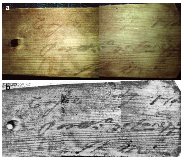
Fig. 6. Tally stick #1 (365nm light source): a - Colour enhanced composite visible image and b - Single band (550nm) composite image
