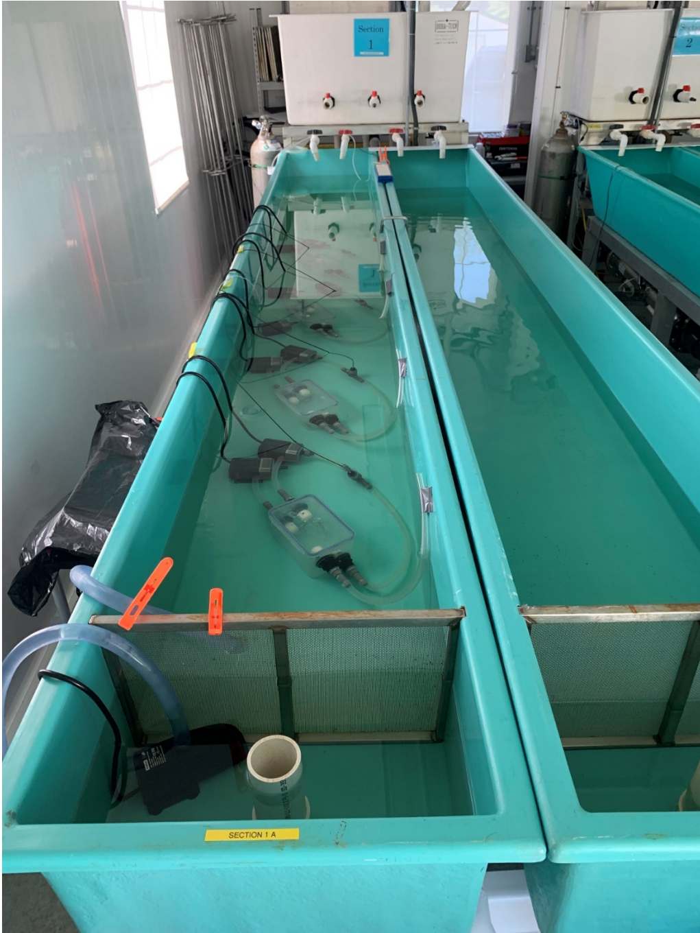
Figure S2. Image of the respirometry chambers placed within the water bath at the WhiteShell hatchery.
