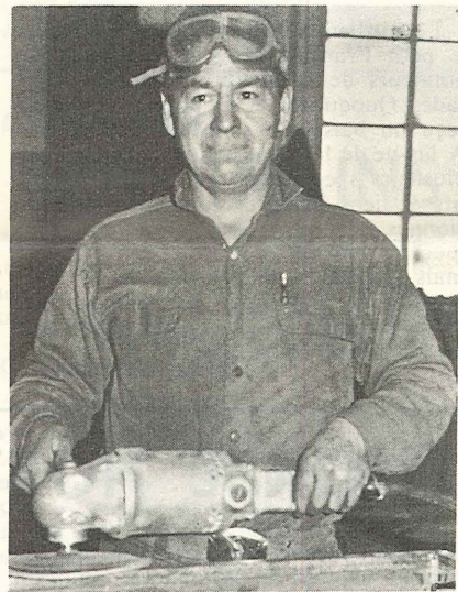
Henry Baptiste grinds a large weldment to produce a smooth finish.
