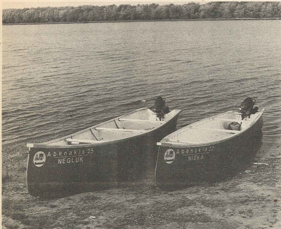
Abenakis freighter canoes, Negluk and Niska, are designed for use on large bodies of water. Made of fibre glass, these craft can carry maximum loads and require minimum maintenance.
