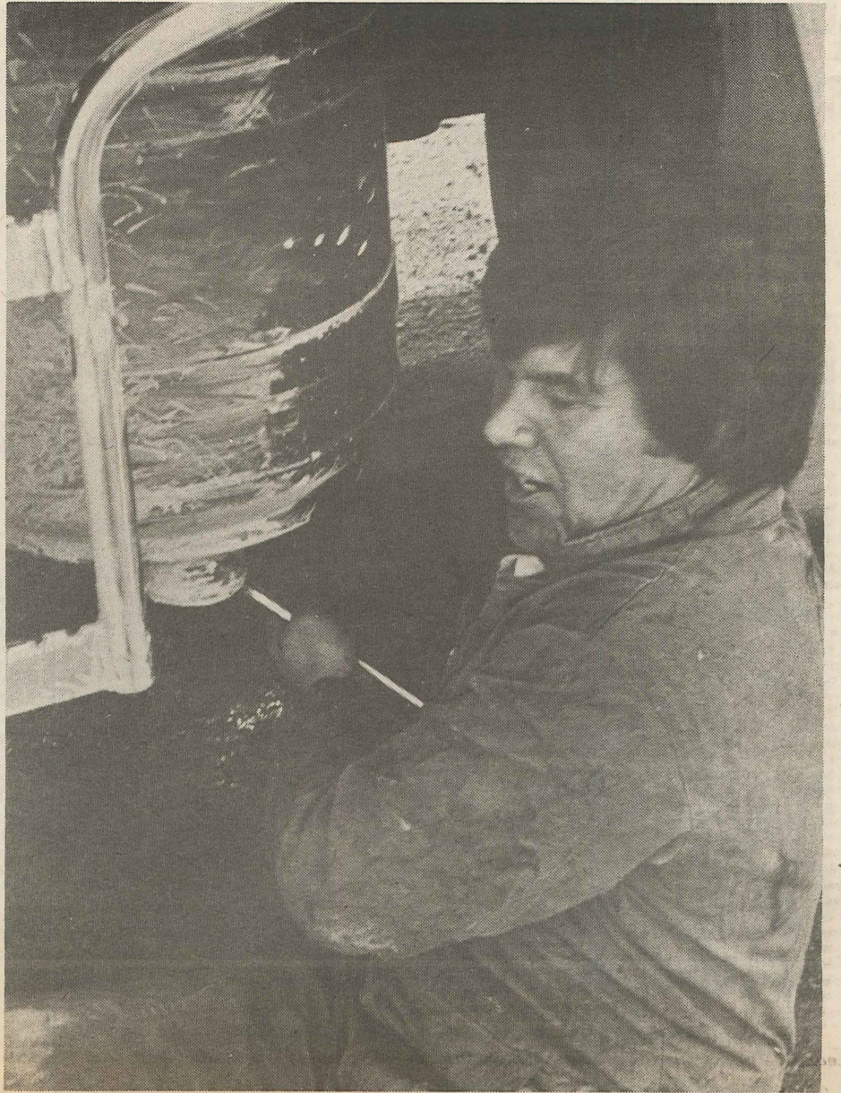
At the roadside, Randy Paul makes an adjustment freeing-up a brake that began to heat-up and smoke.
