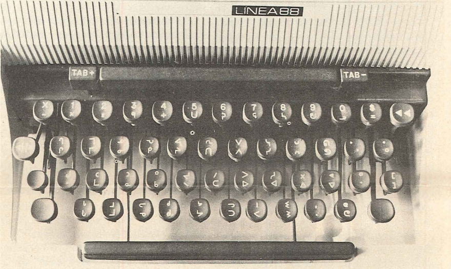
This Olivetti typewriter with the Cree Indian (Western Canada version) syllabic keyboard is the result of months of negotiation between Cree community representatives, Department of Indian Affairs officials and Olivetti Canada engineers. The characters are arranged in vertical rows of similar sounds with the more frequently used syllabics on the second row from the bottom.
