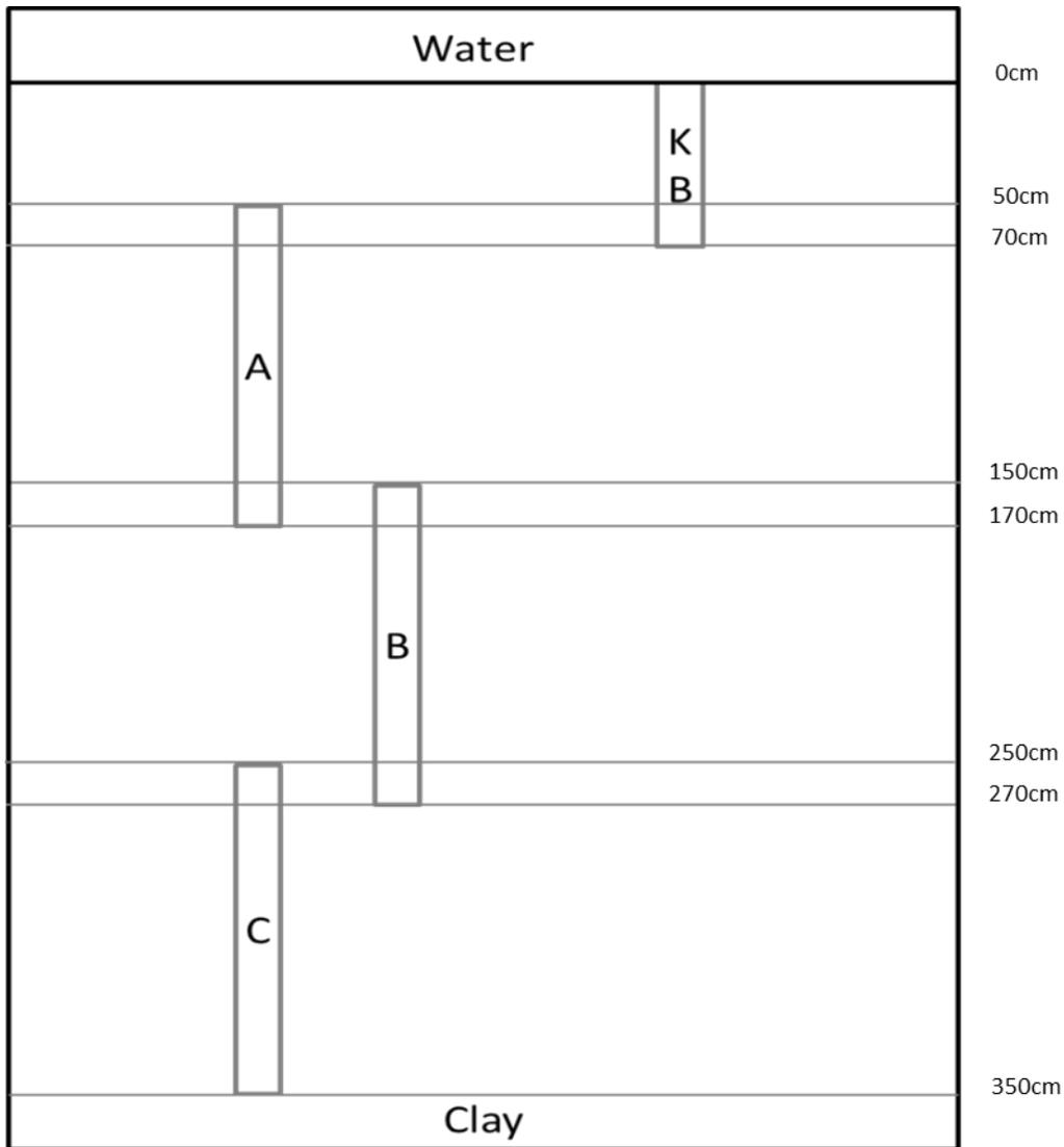
**Appendix X:** Theoretical sampling procedure for extracting successive sediment cores from the lake bottom. The Kajack Brinkhurst core is depicted as KB and the Livingstone cores are depicted as A, B, and C. During field sampling the 20 cm overlap is to enable merging the cores into a single continuous record.
