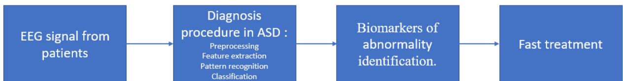
Figure 3-1. The procedure of automated seizure detection (ASD)
