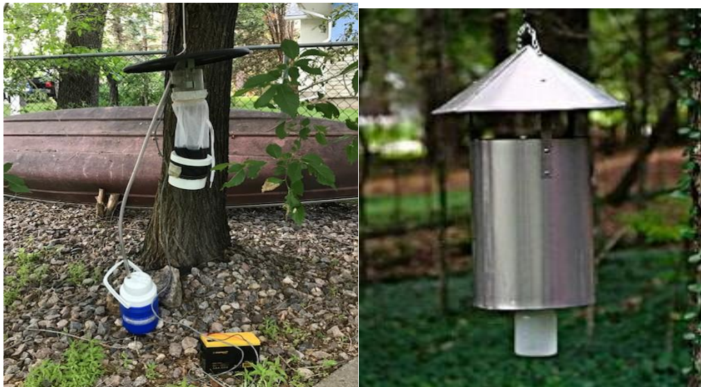
Figure 6. Left: a CDC-light trap baited with dry ice in a blue canister sublimating into CO 2 and operated by a rechargeable 12-volt, 6-amp DC battery. Right: a NJLT with light as a mosquito attractant and plugged directly into an AC power source (John W. Hock Company, Gainesville, FL 2022).
