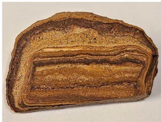
Figure 3: Sample UTE005 cut in half to show internal layering. Sample is 20 mm wide and 14 mm high.
