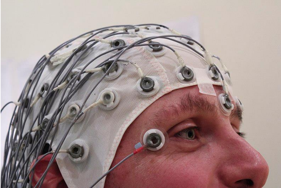
Figure 2.4 EEG electrodes' placement and EEG test device (cap) [Hope12]
