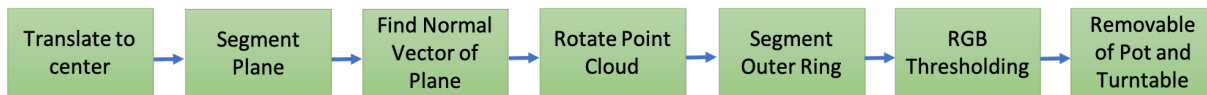
Figure 4.7: The point cloud is translated to center, followed by plane segmentation to identify the turntable points and find the normal vector. Subsequent steps involve rotating the point cloud to align with the positive z-axis and adjusting its position so that the bottom of the point cloud lies on the XY-plane. The next step is segmentation of the outer ring points of the turntable and a color thresholding step to exclude non-plant points, leading to the removal of the pot, turntable points, and any irrelevant points, such as those reflecting the blue backdrop. This is done to refine the dataset for further analysis.
