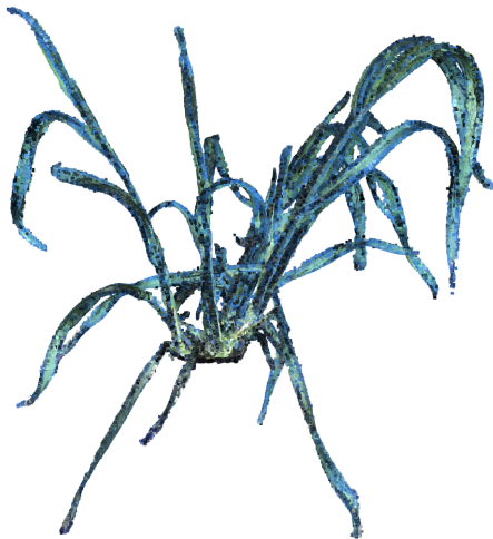
Figure 4.12: A cleaned point cloud following refinement using Meshlab, highlighting the elimination of the pot and turntable to focus solely on the plant. The process encompasses reorienting to align the point cloud with the Z-axis, scaling based on the diameter of the turntable, color-based denoising to emphasize plant-relevant parts, and the removal of all non-plant elements.
