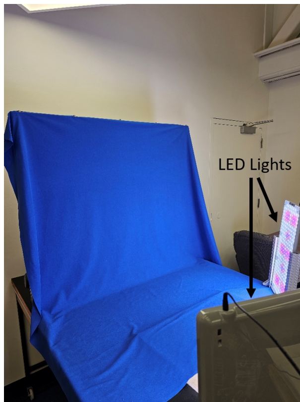
Figure 3.15: The choice of a blue, non-reflective, and uniform backdrop ensures minimal visual noise and optimal focus on the subject. The use of two LED lights, positioned to illuminate the plant subjects, ensures uniform lighting across the subject, minimizing shadows and enhancing the accuracy of images.
