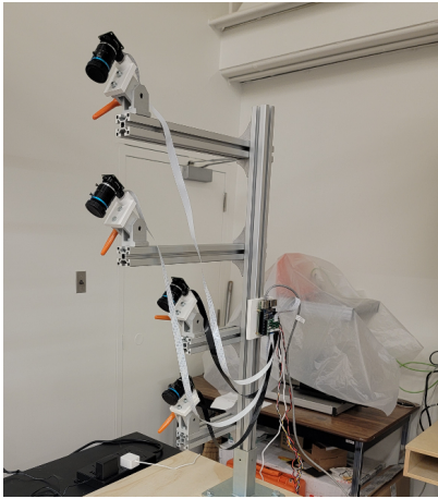
(a) The Raspberry Pi High-Quality Camera connected to the Arducam multi-camera adapter and the photogrammetry rig.
