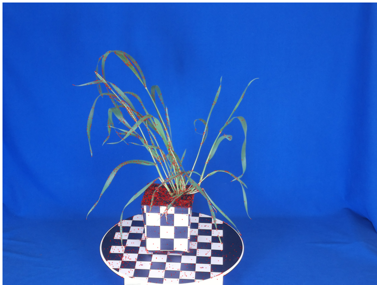
Figure 3.4: Image capture of wheat from the photogrammetry rig. This image shows the key points extracted by COLMAP, highlighting areas for 3D model construction. Features, highlighted as red dots, are essential for matching different images in the dataset, enabling COLMAP to reconstruct the spatial geometry of the scene accurately. The extraction and identification of these points are fundamental, allowing for the precise alignment and stitching of images to generate a cohesive 3D model.
