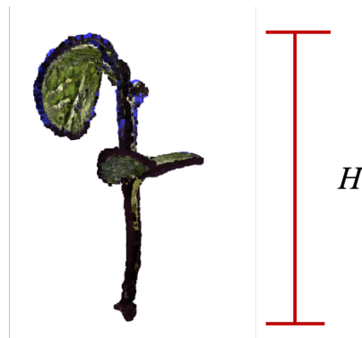
Figure 3.18: Diagram illustrating the method of measuring plant height, with Z_{max} representing the topmost point and Z_{min} indicating the base. This aids in visualizing the procedure outlined in Equation 3.6 for calculating plant height.
